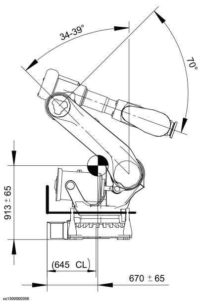
This figure shows the robot in its transportation position.
