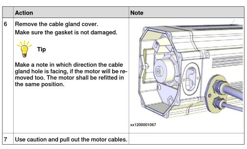
Removing the cable harness - wrist and upper arm
