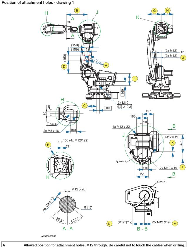
Allowed position for attachment holes, M12 through. Be careful not to touch the cables when drilling.
