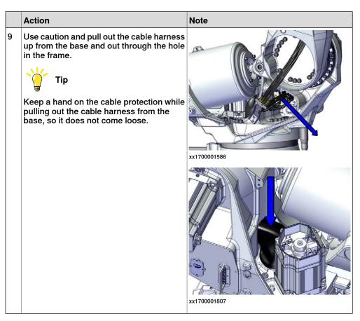
Removing the cable harness in the lower arm
